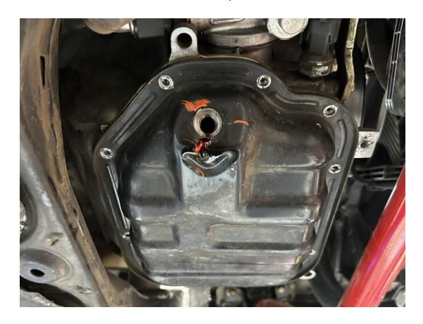
4. Separate the lower oil pan from the upper oil pan. Keep the drain pan underneath, and be prepared for a mess, even though you drained the oil.
