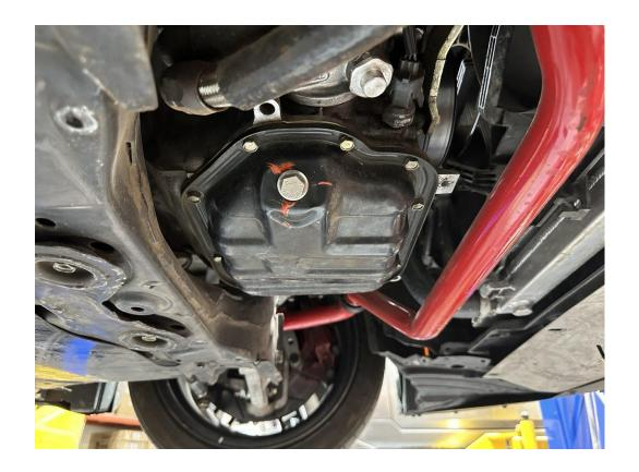
3. Remove the ten 10mm head M6 bolts from the lower oil pan.
