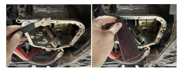
9. You can now start applying RTV to the mating surface of the OEM lower oil pan.
