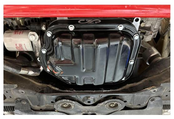
15. Wait 30 to 60 minutes for the RTV to partially set up (depending on ambient temps) and then tighten the lower oil pan mounting bolts in the following order. (Torque spec for the ten M6 bolts is 74-82 in-lb or 8.3 - 9.3 N-m)
