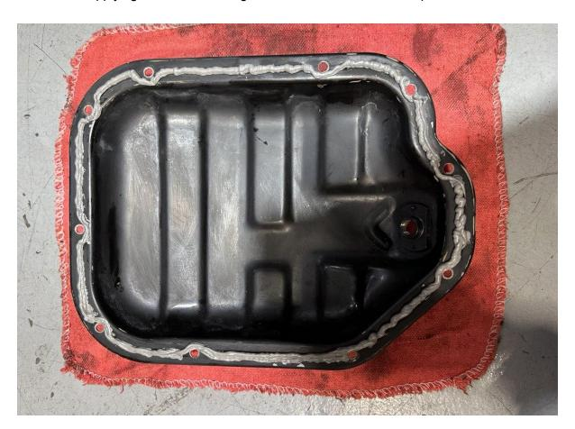
10. Place two or three of the new longer flanged M6 bolts up through the lower oil pan to help align the spacer that we are lowering onto the pan in the next step.
