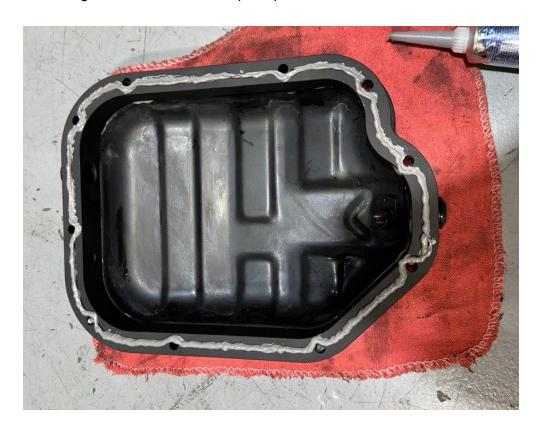
13. Right before installing the lower pan and spacer to the engine, use some brake clean or similar to go over the oil pan mating surface and make sure it is clean of debris and any oil drips. You can see how oil likes to drip from the back edge so make sure to clean it just before you lift the spacer and lower pan into place, or the RTV will not stick and you will have a slow persistent oil leak.
