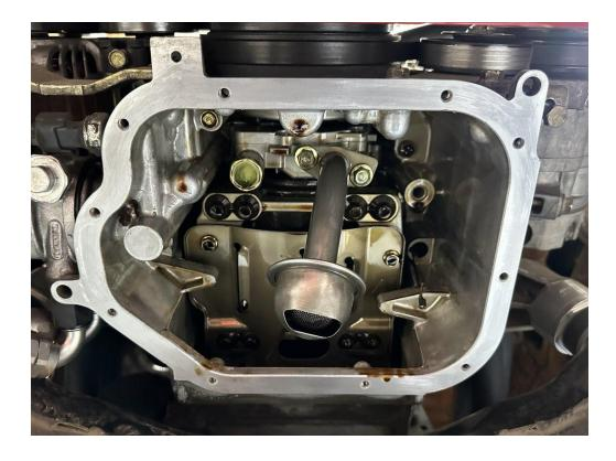
14. Lift the lower pan and spacer sandwich into place and start threading in the two bolts that are aligning the lower pan and spacer. It can help to have a second set of hands at the step to have one person hand thread in all of the bolts while the other holds the spacer and pan in place. Only hand tighten the mounting bolts for now, we will want to wait around 30 to 60 minutes for the RTV to partially set up before we fully torque the mounting bolts.
