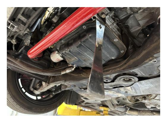
5. Remove the two 12mm head M8 bolts holding the oil pickup strainer.
