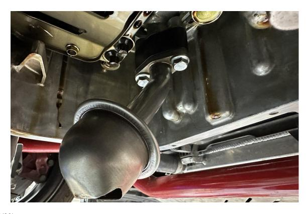
8. Clean both the mating surfaces of the upper and lower oil pans of the old RTV sealant using a razor and some Scotchbrite pads or similar.
